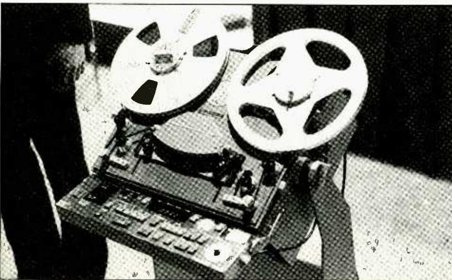
Nagra T-Audio twin capstan multiformat recorder
