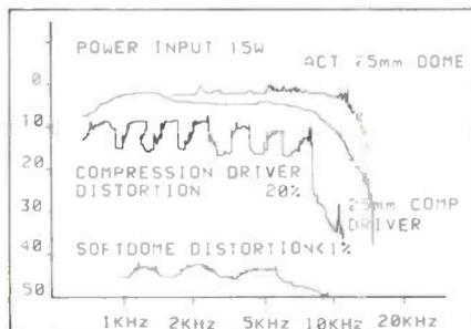
Soft dome design produces less than one tenth the amount of distortion of the conventional compression types.
