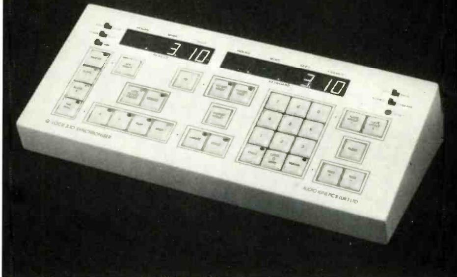
locate points; record/offset/locate memory frame trim facility; user definable preroll and instant replay; full transport remote controls; high speed tachometer processing eliminates need for tape-to-head contact in wind; Q-Link feature allows linkage of two more Q.LOCK systems for control of five machines or control by external computer command source—many interfaces available.
