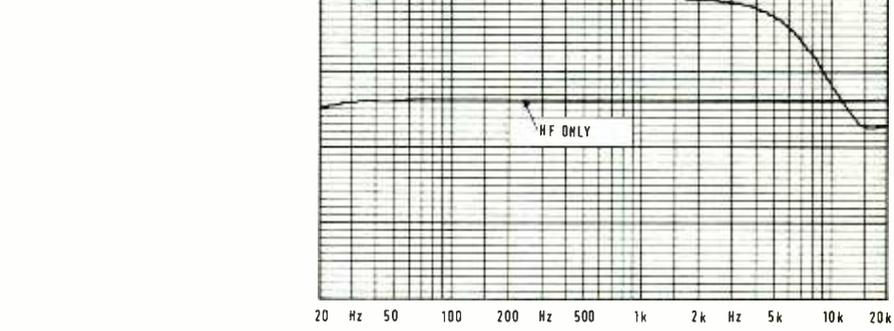
FIG.3 dbx 902 DE-ESSER HF RESPONSE WITH FREQUENCY CONTROL
