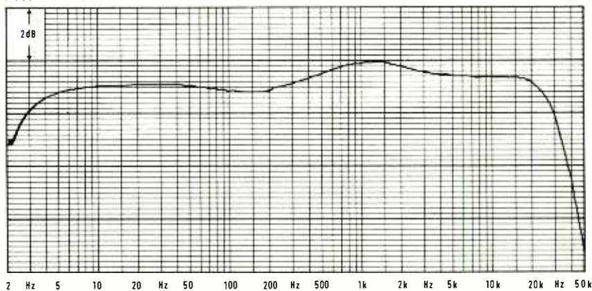
FIG. 17 dbx 905 PARAMETRIC EQUALISER RESPONSE WITH THREE SECTIONS IN NOTCH MODE
