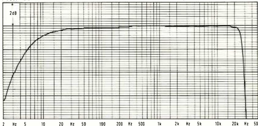
FIG.2 FOSTEX B-16 REPLAY EQUALISER
