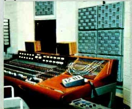
... extended low frequency response can be achieved simply by spacing panels away from walls. . .
