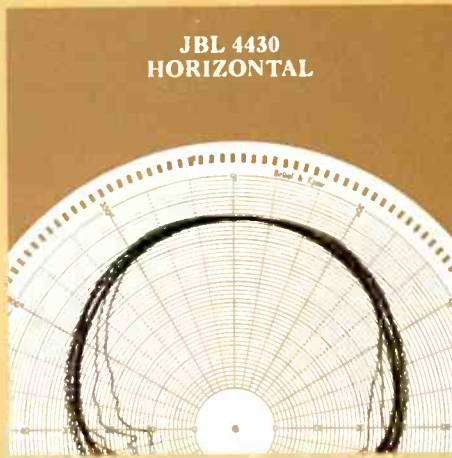
Polar response of a 4430 studio monitor:
