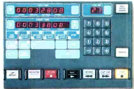
ATR-124's Multi-Point Search-To-Cue (MPSTC). Provides 100 cue locations.
