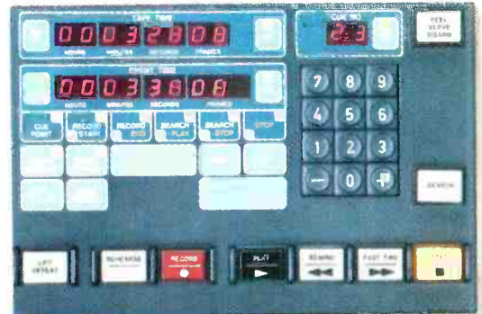
ATR-124's Multi-Point Search-To-Cue (MPSTC). Provides 100 cue locations.
