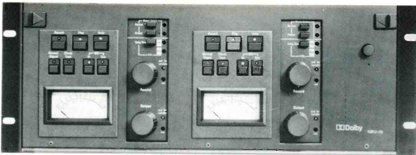
Dolby NRU 10. A new two-channel audio noise reduction unit for videotape recorders.
