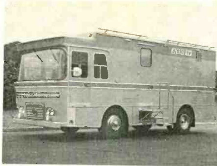
Left: The latest BBC television outside broadcast for Open University which has been designed and built by Link Electronics. The vehicle is part of the Open University's plans to go over to full colour and is engineered to a complete colour television studio and control room facility.
