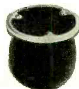
4021 OMNIDIRECTIONAL Moving coil 40 Hz - 12 kHz Impedance: 30Ω Output: -80 dB ref 1V/dyne/cm 2
