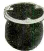
4021 OMNIDIRECTIONAL Moving coil 40 Hz - 12 kHz Impedance: 30Ω Output: -80 dB ref IV/dyne/cm 2
