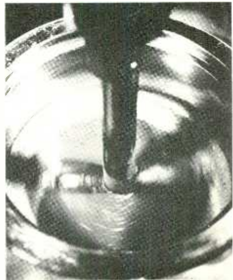
Making the iron oxide dispersion.
