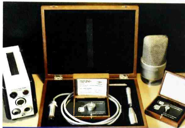
Reference valve type B&K, together with modified Neumann M50
