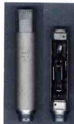
Outside and inside view of the MKD MV101 calibration microphone
