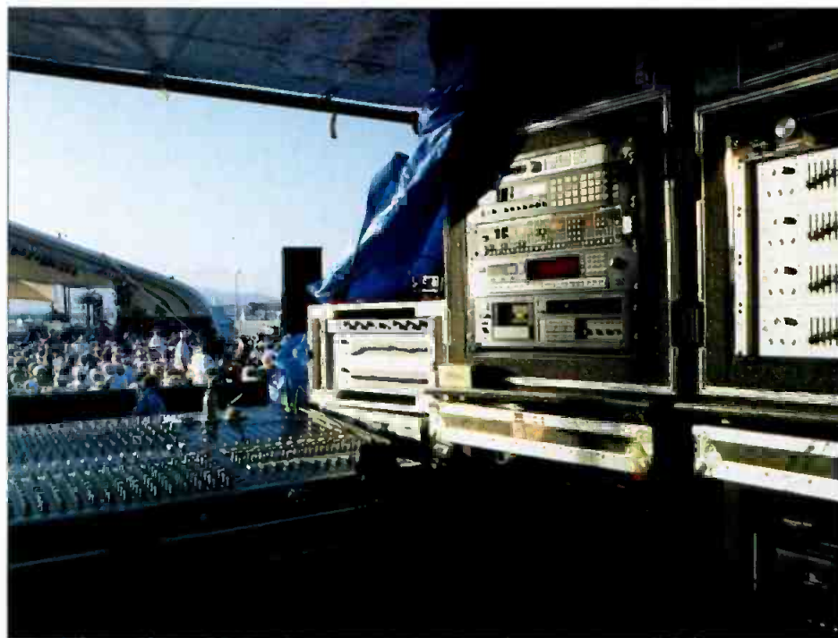
The FOH mix position featured a 32 x 12 ATL console, used to handle program bus assignments for both stage monitors and main systems. The (4) Industrial Research Products T.E.Q. graphic equalizers in the foreground were assigned to onstage foldback mixes.
