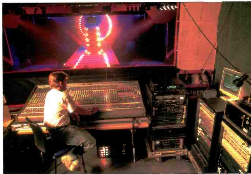
The control room housed a 40-channel console with 22 separate controllable outputs, along with a 1/2-inch 16-track, which contained all of the music, effects, film sound and voice-over elements, each recorded on separate channels and pre-mixed for each of the loudspeaker chains.
