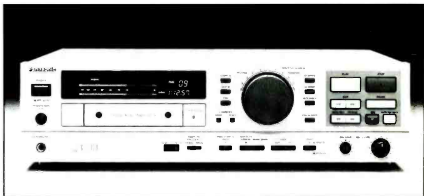
The Panasonic SV-3700 was the reference machine to test other DAT players and their treatment of the SCMS scheme.
