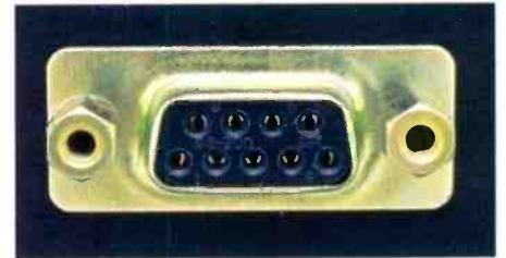
9-pin serial port for control by Sony video editors BVE-9000 or BVE-900.
