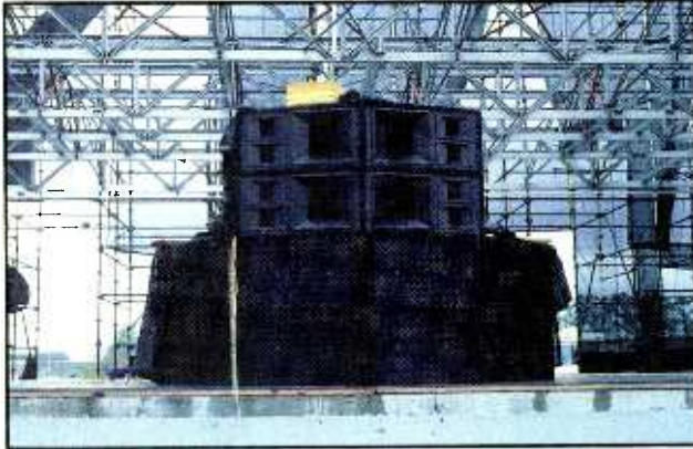
Photo 11. After proving that electronically controlled speaker systems could be accepted in the marketplace, system manufacturers worked on development projects for larger, arrayable components for sound reinforcement use. Shown here, the first outdoor field test of the Renkus-Heinz MR-1/LR-2M system (on stage at Irvine Meadows Amphitheater in Southern California).
