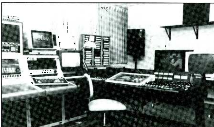
Photo 4. An audio-for-video-post suite at Soundelux in Hollywood. Notice that the AMS AudioFile is built into the mixing console.
