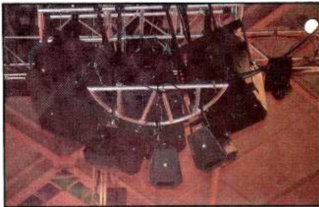
Photo 12. Manufacturers intent on producing large-scale systems for the professional market must offer enclosures that are easy to use in arrays in hanging situations. Shown here, Apogee Sound's 3X3 and AE-5 enclosures in an array by Burns Audio at the 1988 Democratic National Convention.
