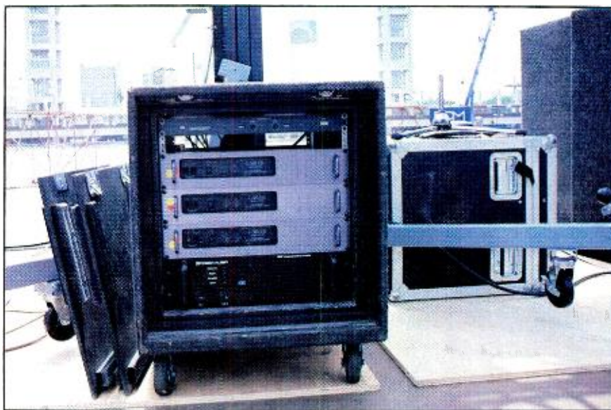
Photo 2. Compact rack for powering sidefill monitor enclosures includes amplifiers from Carver and Crest.
