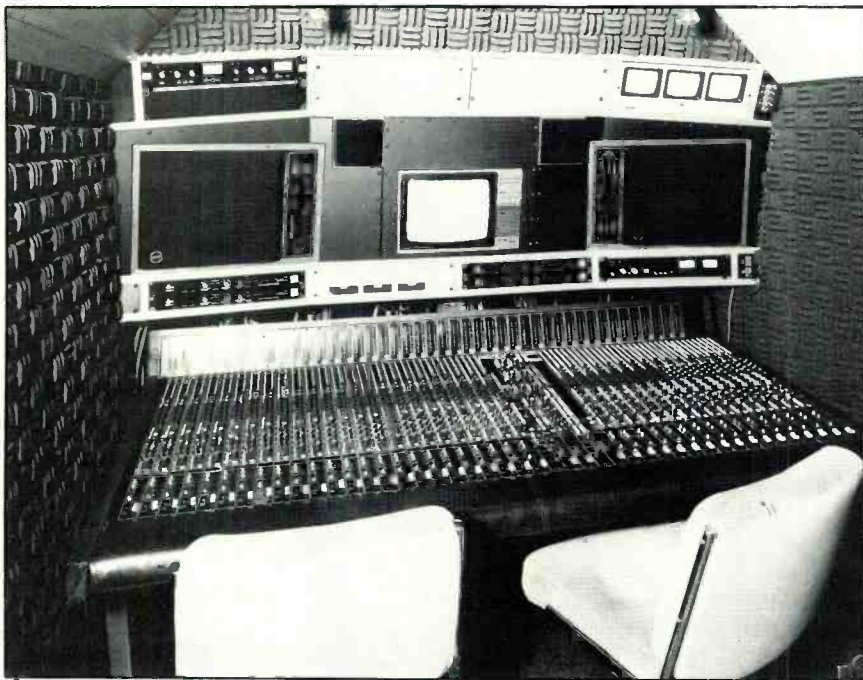
The Metropolis van features a Harrison 40/32 console, Tannoy and Auratone monitors, dbx 160, 160X and 162 compression and limiting and communication facilities.
