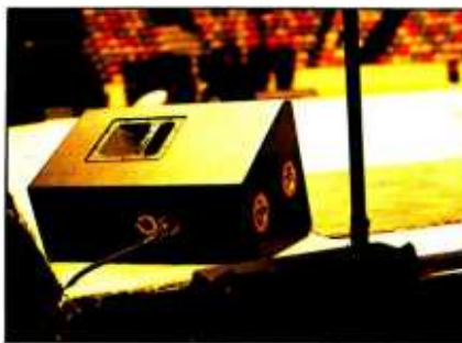
Figure 11. Four Meyer UPA-1A angled speaker enclosures serve as stage area monitors for the vocalists.
