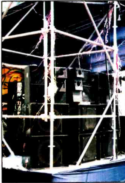
Modular stacks at the Jambalaya Jam in Philadelphia. A 2-box, 4-way system uses the Joe's Slide-Align to align the high and super-high horns to the 12-inch speakers in the same cabinet.
