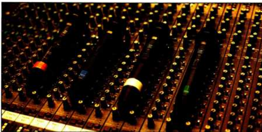
Figure 12. Shure's new wireless microphone transmitter for hand-held use with SM87 head capsule. (Units are resting on Yamaha PM-3000-40 mixing console.)
