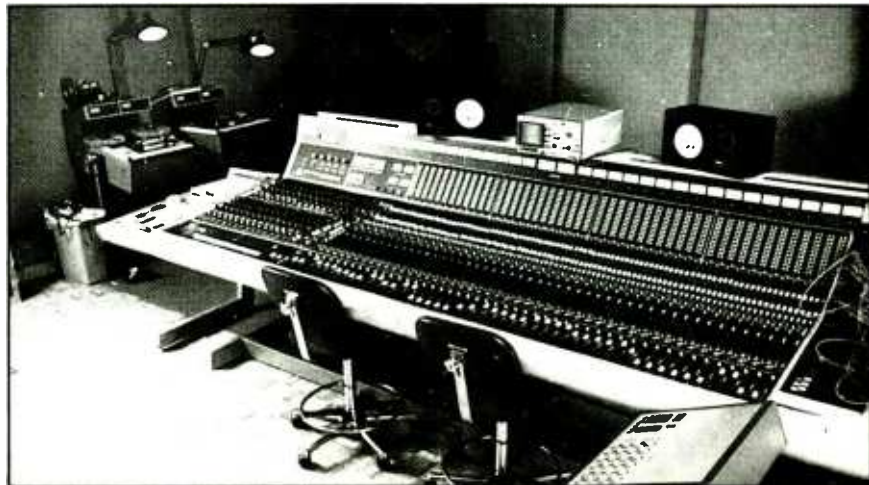
Prairie Sun's Studio A features a Trident TSM 48x32x80 console, Sturmer and Ampex tape machines, and Q-Lock synchronization. During a typical session, tracking and overdubs occur in Studio B, with mixing in Studio A.
