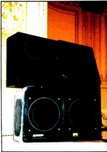
House sound system for Judy Collins' and Arlo Guthrie's performances at Carnegie Hall. Note that the left-hand mid-high cabinet wears lenses to increase the dispersion of the high and super-high horns, while the right-hand box has been tilted at a 30° angle to cover the balconies.
