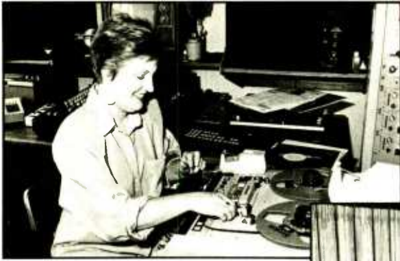
Selected music cues can be transferred to 1/4-inch tape from vinyl albums, Compact Disc or reel-to-reel masters prior to fine tuning timings to match picture. The final edited master would then be transferred to a time code-striped 1/2-inch 4-track, or bounced up directly to the 16- or 24-track multitrack master prior to the sweetening and remix session.
