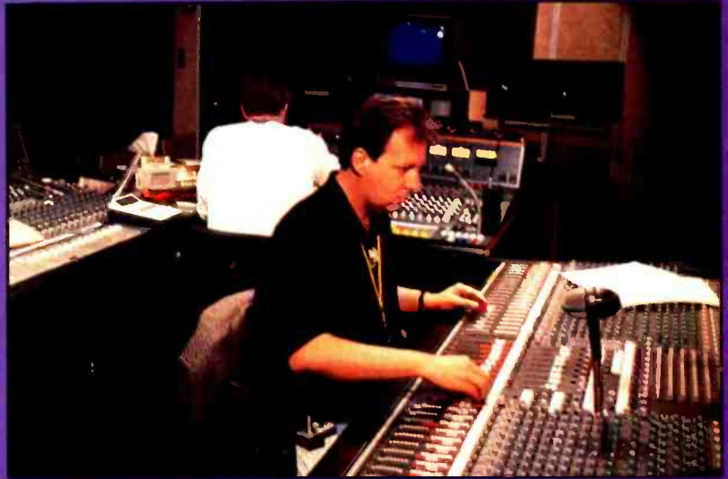
The main audio control booth at Fox Television Studio 4, used for the live stereo broadcast of The Late Show starring Joan Rivers, features two consoles on L-shaped Neue model 4875 board (left and center) at which assistant engineer Ron Worrel handles the master stereo broadcast mix and the submixing of dialog sources. At the Yamaha PM3000 console (right), production engineer Thom Wilson handles mic and line-level sources from the house and guest bands. Inputs to the larger submixer section include desk and audience mics, boom mic, radio mics and audio outputs from various VTRs. The Soundcraft series 200D above the side console accommodates additional inputs.
