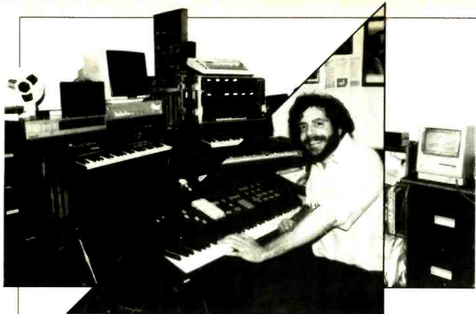
The author in his personal-use studio during recording of The Celtic Macintosh project, surrounded by the various MIDI-equipped sequencers, keyboards and signal processors. From left-to-right: a Panasonic PV-1231V VHS videocassette recorder used during the PCM-encoded mastering stage; Auratone 5C Sound Cube close-field monitors; a Sony PCM-701ES EIAJ-format digital processor; Taxan video monitor (for use with the 701); Kurzweil K250 digital synthesizer; Yamaha DX-7 FM synthesizer; TOA model D-4 console and D-4E expander module; Lexicon PCM-70 MIDI-capable digital delay and reverb processor; Southworth Music System's MIDI interfaces and companion Apple Macintosh PC.
