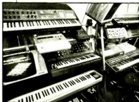
The keyboard array at the second studio includes (left-to-right): a Fairlight CMI series II, PPG Wave 2.2, Roland SBX-80 time code-to-MIDI converter, Minimoog, Oberheim Expander, Roland MKS-80, Yamaha DX-7 and Sequential T-8 synthesizers.
