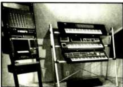
In the rear of the room are located a separate keyboard submixer, PPG Waveterm controller and VDU (left) and the facility's main keyboard array: a Sequential 2000, E-mu Systems Emulator II and a PPG Wave 2.2.
