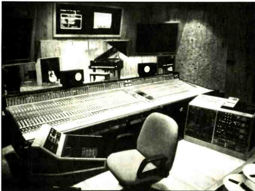
Royal Recorder's overhead video monitors in background display stored settings and the 80-input Solid State Logic console with 64 mono channels, eight stereo channels and primary/total recall.
