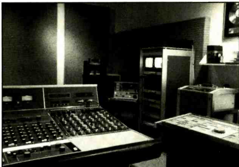
Available for use throughout Sterling Sound for disc and CD mastering are a Sony DAE-1100 digital editing system (right) and a Mitsubishi X-86 PD-Format digital 2-track (to the right of main equipment rack).
