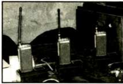
Figure 4. Pace Landmaster III radio communicators were specified to facilitate sound-crew communications during setup.
