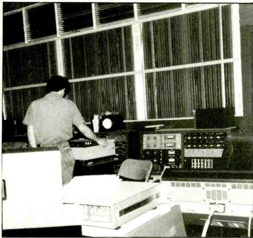
To the right of the console during the 72-track AT&T digital remix sessions were located three Sony PCM-3324 multitracks synchronized via their individual remote control units. The pair of PCM-3324s pictured right are owned by Master Sound Astoria, and the unit to the left was rented for the session from AT Scharff, New York.
