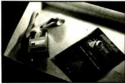
Figure 3. The conductor in the orchestra pit communicated with the sound mixing positions by means of a handset and belt-pack.
