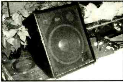
Figure 12. JBL model 4602 compact floor monitors were supplied by the Civic Auditoriums' sound department.
