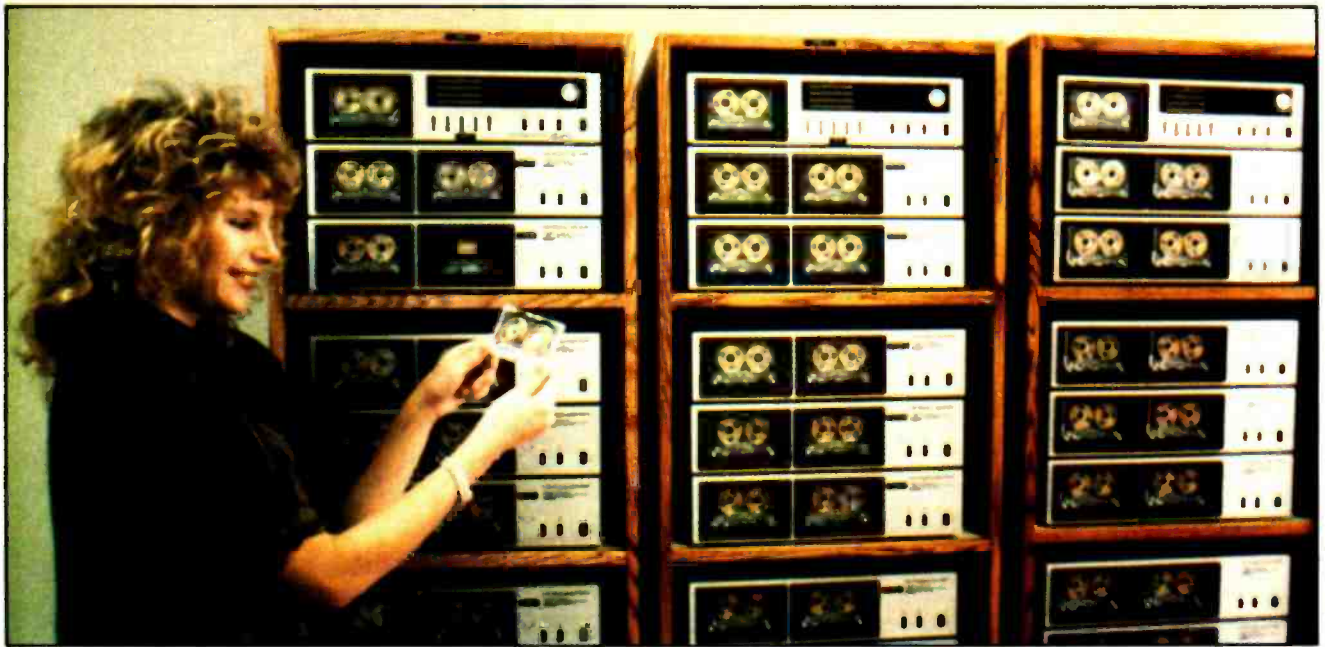
A KABA in-cassette duplication system capable of real- and 2-times ratios, installed recently at AT&T, Los Angeles.
