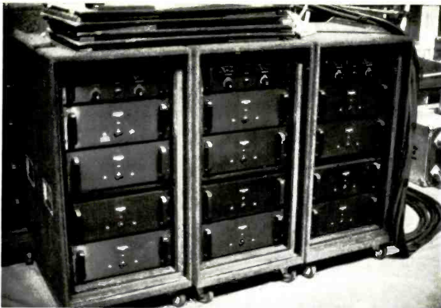
Figure 20: SSG amplifier racks housed three 1,200-watt, one 800-watt one 400-watt specially-modified Cerwin-Vega power amps; 300 watts of power is available to each 18- and 15-inch speaker.
