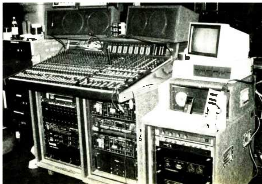
Figure 5 : Stage-right keyboard mix position — Gamble SC-24-24-II console, stereo monitor loudspeakers, and an IBM personal computer. (This position manned by David Bowers.)
