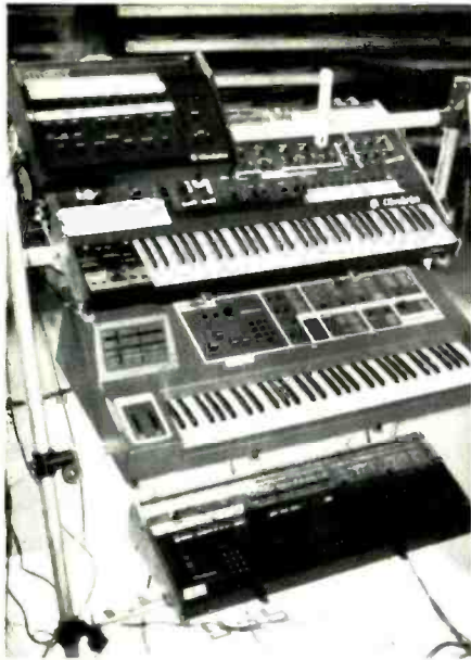
Figure 6: Stage-right auxiliary keyboard rack, where MIDI-connected instruments for David Paich include an Oberheim DSX, Oberheim X-Pander, and an E-mu Systems Emulator II.
