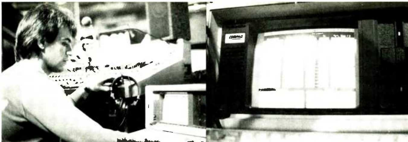
Figure 3 (left): A Compaq personal computer located at the stage left submix position. Each song in the show has a "menu" showing which instruments are in use, as well as MIDI patches. Figure 4 (right): The Compaq display screen, showing an informational display designed by keyboard expert Ralph Dyck.
