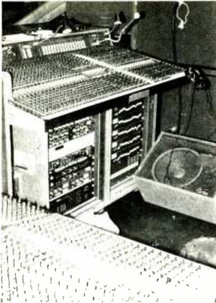
Figure 13: The monitor mixing area, downstage right: Gamble SC40-16 and Gamble SC32-16, handled by Dirk Schubert and Alan Bonomo.
