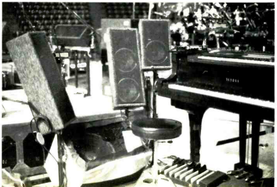
Figure 9: David Paich's stage monitors: the small enclosure next to the piano keyboard carries a vocal mix only. A stereo keyboard mix is also available from the mini-columns.
