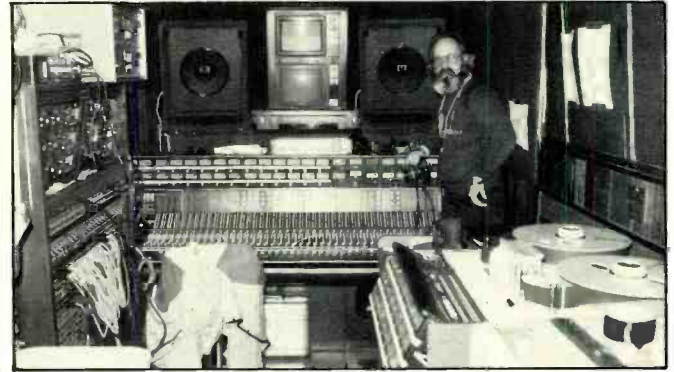
RECORD PLANT/NY: two Ampex MM1200 24-track and Ampex ATR100 2- or 4-track tape machines; custom API 44x44x24 console with built-in API 560 limiters; monitors by Westlake, modified and powered by Bryston 4B amplifiers; UREI and Teletronics limiters on truck, and other equipment supplied as needed. 321 W 44th St., NY, NY 10036. (212) 581-6505
