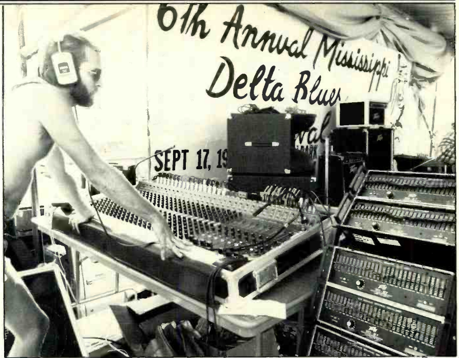
Monitor mixing position, with outboard signal-processor and EQ rack, and cross-stage monitor cabinets.
