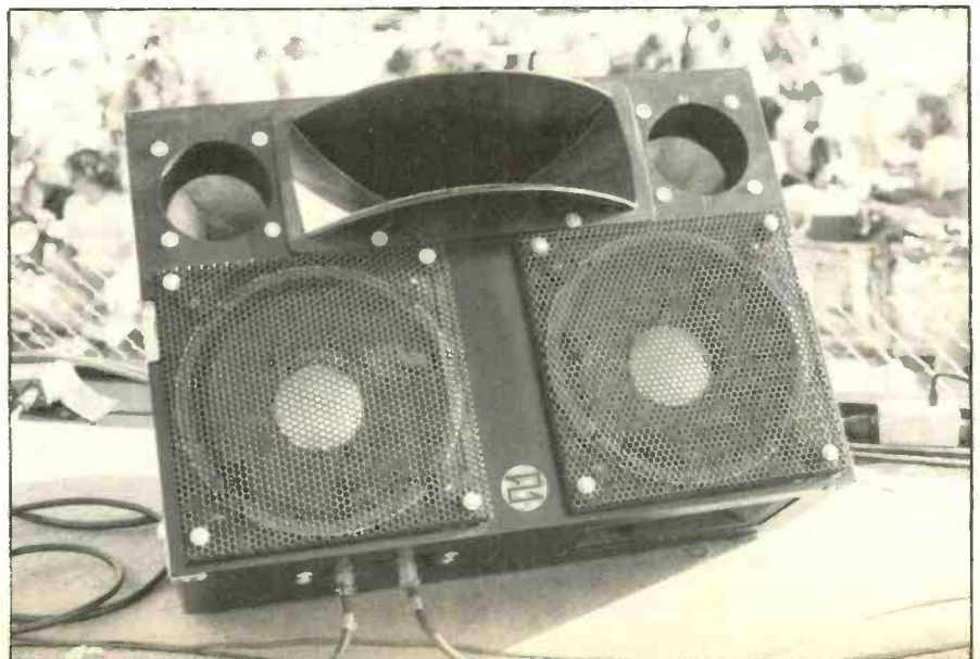
Figure 7: Vocal floor slants comprised an EAW 2-12 cabinet loaded with JBL 2202 12-inch cones, and a 2441 compression driver.
