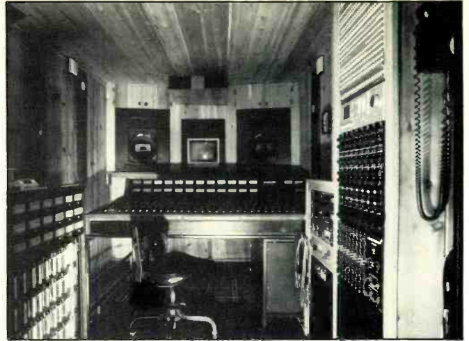
TIM PINCH RECORDING: AMEK 44 input 28/24 customized console; Ampex MM1200 24-track and AG440C 4- and 2-track tape machines; monitors are Altec 604-E with Mastering Lab crossovers and Auratones; video equipped. 6600 San Fernando Road, Glendale, CA 91201. (213) 507-9537.
