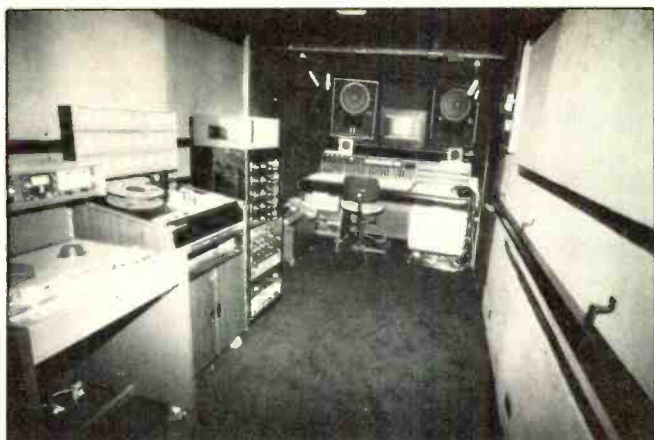
ROCSHIRE RECORDING: Mobile 1 is equipped with 3M M79 24-track and 2-track, and a Sony PCM-1610 digital processor; custom 32-input API console; monitors are modified JBL 4320s; full outboard rack of signal processors. 1240 North Van Buren, Anaheim, CA 92807. (714) 632-5046.
