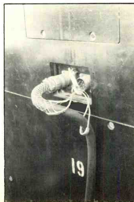
Figure 3: Back of the CS-3 two multipin connectors, and a hook for cable strain-relief.
