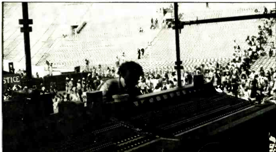
Figure 6: A pair of Yamaha PM-2000-32 consoles provided a total of 64 mike channels for the main-stage sound mix; house engineer Ed Wynne at the controls.
