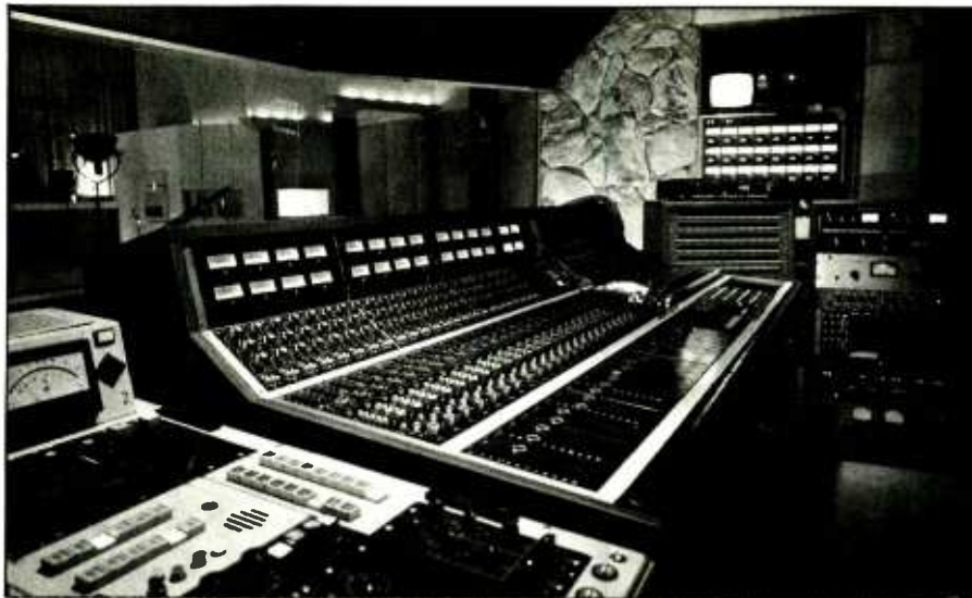
Control room equipment centers around an API 2488 console, Studer A800 and Lyrec TR532 multitracks, Studer, MCI, and ReVox mastering machines, Westlake HR-1 monitors, and dbx, UREI, Eventide, Lexicon, and Orban outboard signal processing units.
