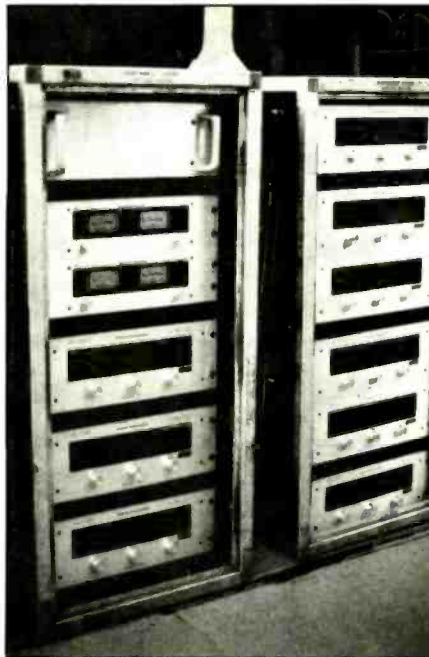
Figure 5: Northwest amplifier racks contain Marantz Model 510, 240, and 140 units housed in a rigid external metal frame, with impact-resistant front, side and rear panels.
