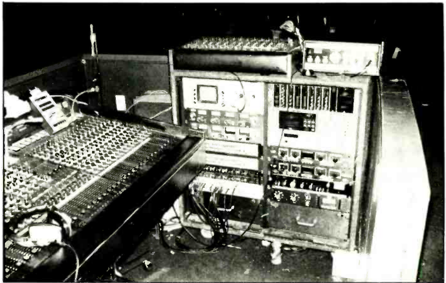
Mixing booth setup for Linda Ronstadt Tour, September 1982. Main sound contractor for the tour was Showco, who supplied a custom-designed 30-in/8-out stereo console, Kelsey 12/2 keyboard mixer, Sound Workshop 12/8 effects subconsole, and various effects units. Stanal Sound also furnished an outboard rack containing a Yamaha Q1027 graphic equalizer, dbx Model 162 compressor-limiter, Clear-Com KB-115 intercom remote station, Yamaha M406 submixer, and crossover units.
