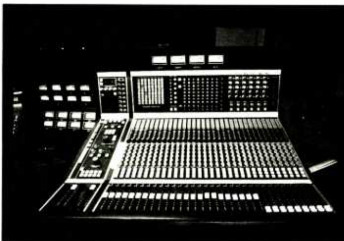
Custom-designed 40-input sub-console interfaces directly with the main SSL board, and provides separate monitor and fold-back mixes. Six discrete headphone send busses are available.
