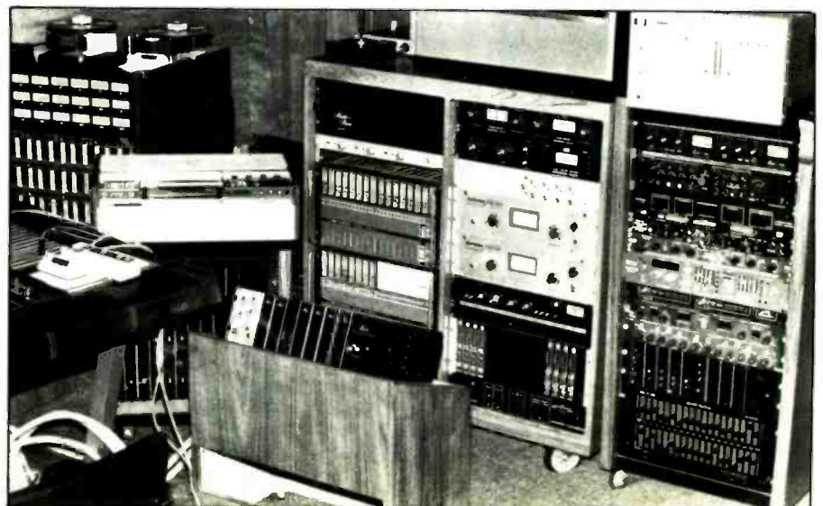
The two digital audio processors — dbx Model 700 and Sony PCM-1610, plus companion U-Matics — used for comparison evaluations at Crescendo.
