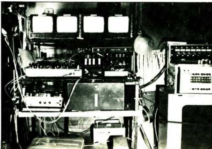
Interior of Jim Webb's sound van, with video monitors providing a through-the-lens view of the scene being recorded on the Stephens 8-track (right).
