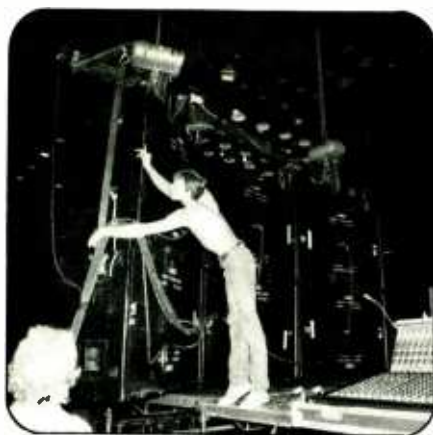
Figure 2: Jands "Concord" cabinets mounted together to form a hanging array.
