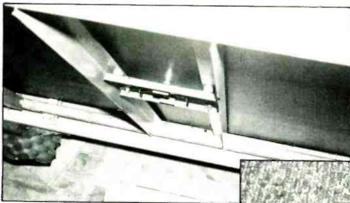
Top View of drive coil assembly, showing mounting for drive magnet and packing washers.
