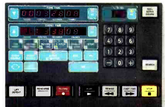
ATR-124's Multi-Point Search-To-Cue (MPSTC). Provides 100 cue locations.
