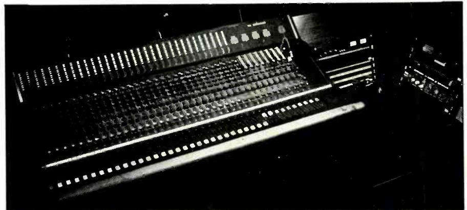
Figure 2: TFA/Soundcraft Series III house mixing console, equipped with 32 inputs, eight subgroups and two main plus eight effects outputs.
