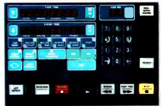
ATR-124's Multi-Point Search-To-Cue (MPSTC). Provides 100 cue locations.
