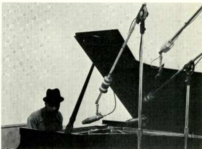
Three microphone set-up at Sigma, Philadelphia
