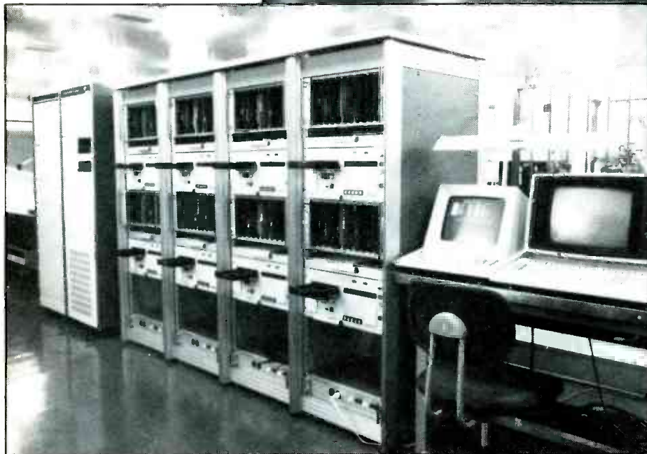
Right. High speed visual inspection machines developed by JVC for detecting inclusions, spots and scratches etc.
