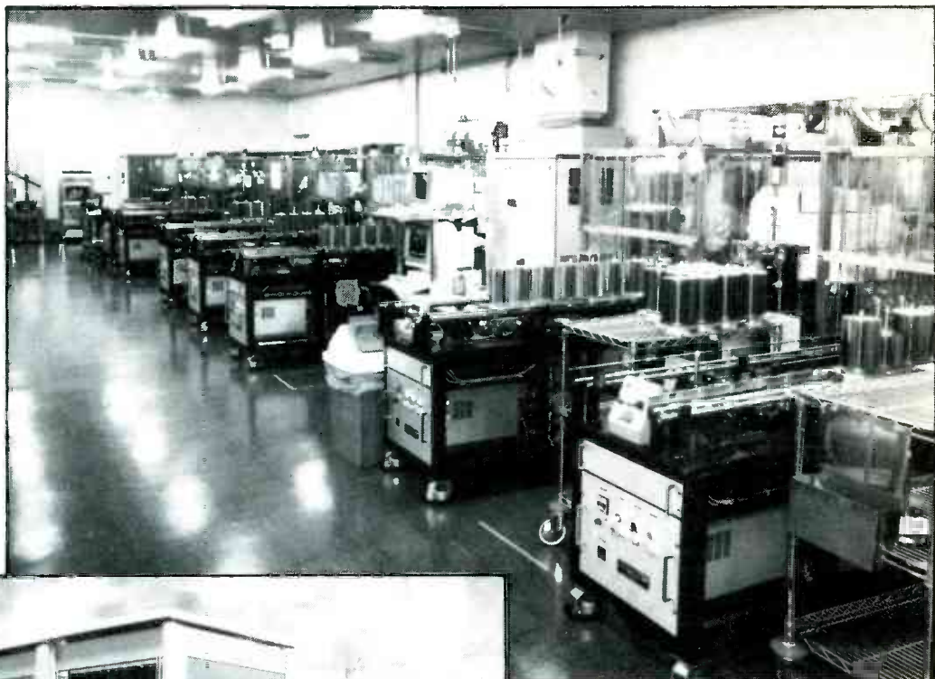
Right. High speed visual inspection machines developed by JVC for detecting inclusions, spots and scratches etc.
