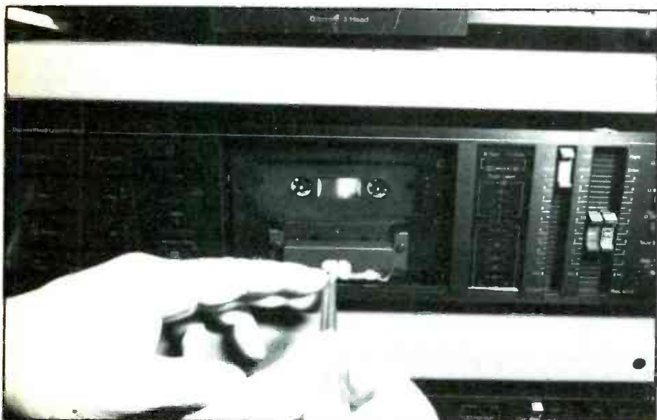
Adjustment of azimuth on the BX300E
