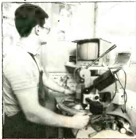
Centring: the centre hole is cut
