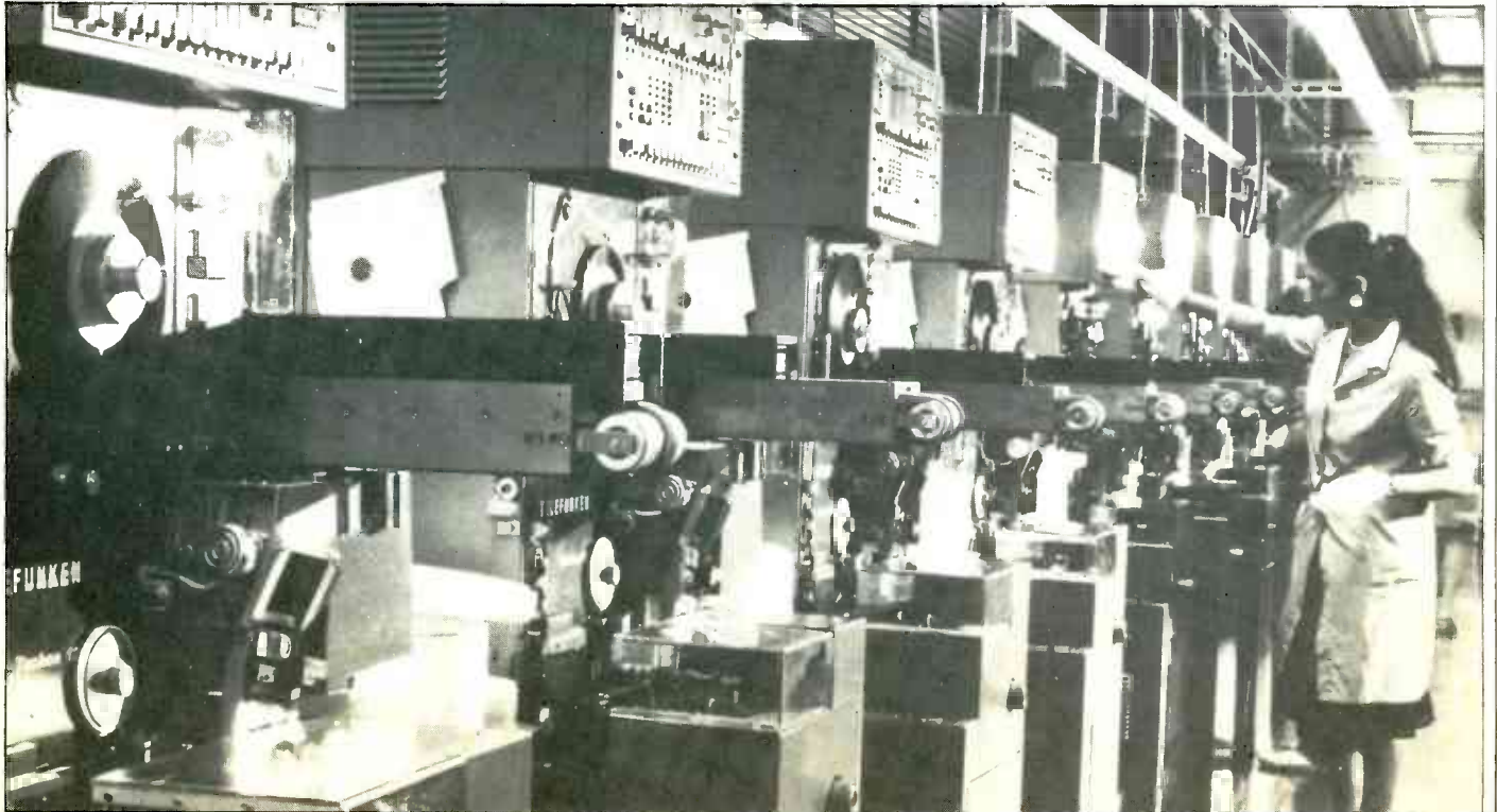
Cassettes being loaded automatically with magnetic tape
