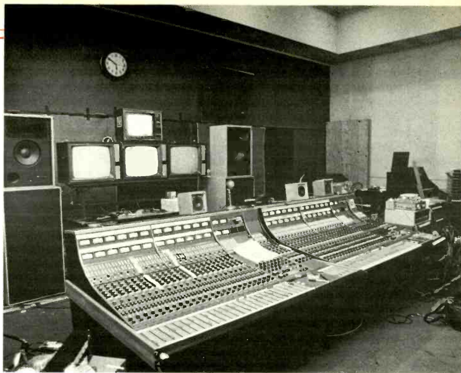
The two 24-channel Neve boards and the ACD Monitor System used in the studio.
