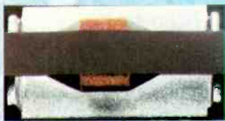
TDK dual spring pressure pad and tape in cassette.
