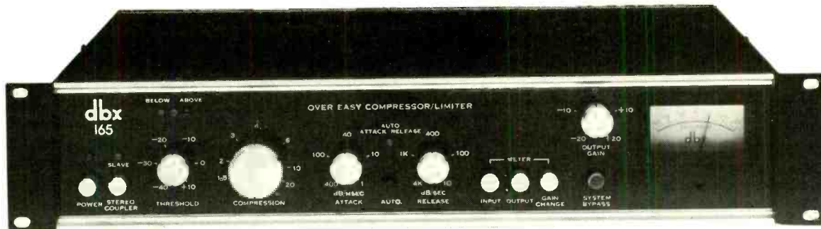
The dbx 165 is our top of the line, and it's as flexible as you want it to be. Attack and release rates can be adjusted manually or automatically. Both threshold and output levels are adjustable. And the 165 can be strapped for stereo, with a front panel master/slave switch for easy operation.
