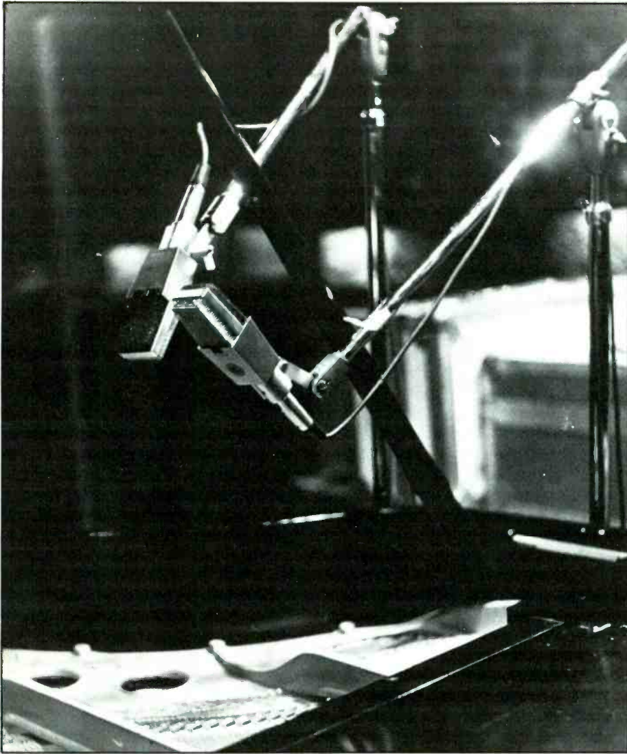
Photo depicting the "X" configuration technique used for piano miking.
