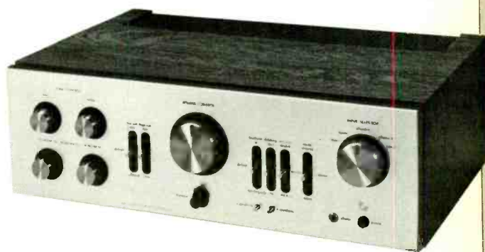
Luxman L-80V integrated stereo amplifier. 50 watts minimum continuous power per channel, with total harmonic distortion no more than 0.08 per cent, both channels driven simultaneously into 8 ohms, 20 to 20,000 Hz. Frequency response, 10-50,000 Hz, within 1 dB. Phono S/N better than 77 dB (re: 10 mV input). Bass and treble controls each have 3 turnover frequencies; high and low filters each have 2 cut-off frequencies. $475. (Luxman L-85V, similar except 80 watts per channel, $765.)
