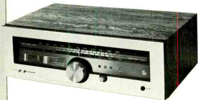
Luxman T-88V AM/FM stereo tuner. Our least expensive tuner, yet includes FET front end with four-section tuning capacitor. Linear-phase ceramic filters in IF section. Features include FM interstation-noise muting, variable output level control and oscilloscope jacks for viewing multipath distortion, etc. Usable FM sensitivity; 2 microvolts (11.2 dBf) IHF and 2.8 microvolts (14.1 dBf) for 50 dB quieting. Stereo separation: 43 dB at 1,000 Hz. $345.00
