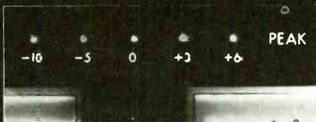
5 LED peak level indicators help eliminate distortion.
