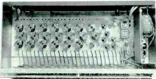
Klark-Teknik DN27: Internal view.
