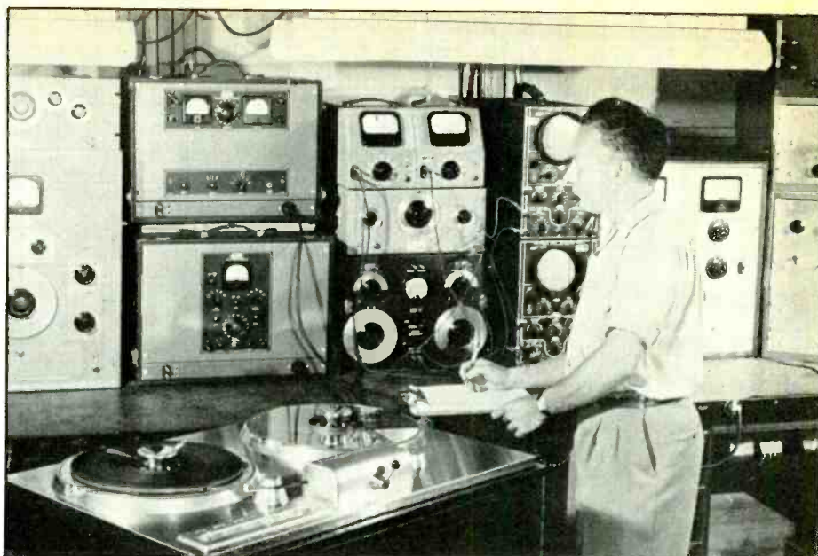
Project engineer Harold Lindsay and the Ampex 200's which were closely modeled after Mullin's Magnetophons.
