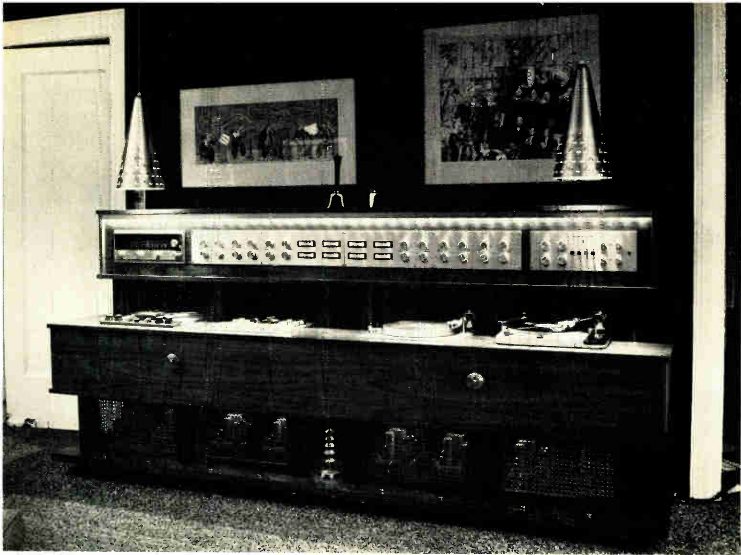
This nine-foot cabinet was constructed in walnut by Russell Clancy (who authored "The Joys of Shopping for Stereo" in this issue). Controls are mounted on the top deck; the main deck contains (right to left) Thorens' TD 124 turntable, with Grado Lab Series arm and ADC cartridge, the Rek-O-Kut B-12H turntable with Grado arm and Lab Series cartridge, a switching panel—mostly of AC switches, and an Ampex 960 tape recorder. The lower deck houses eight Marantz 30 watt amplifiers. Four of these feed five ranges of speakers on each stereo channel with the limited signals they receive from electronic crossovers. Also included are McIntosh tuner (far left, top deck) and Knight TV audio tuner (switch panel, main deck).
