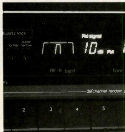
The RF and IF bandwidth indicators (center)
