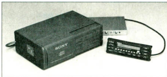
Sony's new CD changer system consists of the small changer mechanism, the wired remote commander, and an optional hideaway chassis containing the tuner circuitry. Another option (not pictured) is the XK-8D half-DIN cassette deck ($300). A second hideaway box houses control circuitry for the changer and is the connecting point for the remote, the tuner box, and the deck.
