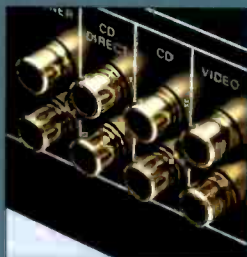
Gold-plated input jacks on the Citation twenty-one preamplifier provide reduced signal loss and improved long-term conductivity.
