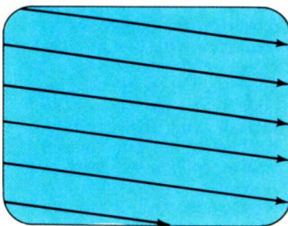
Fig. 1. A TV picture is made up of a series of nearly horizontal scan lines traced from top to bottom.
