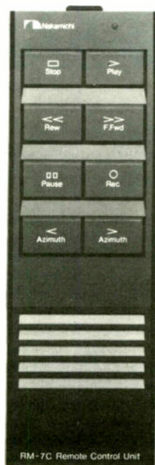
THE CR-7A'S REMOTE HANDSET PROVIDES CONTROLS FOR ALL BASIC FUNCTIONS, INCLUDING PLAYBACK AZIMUTH ADJUSTMENT
