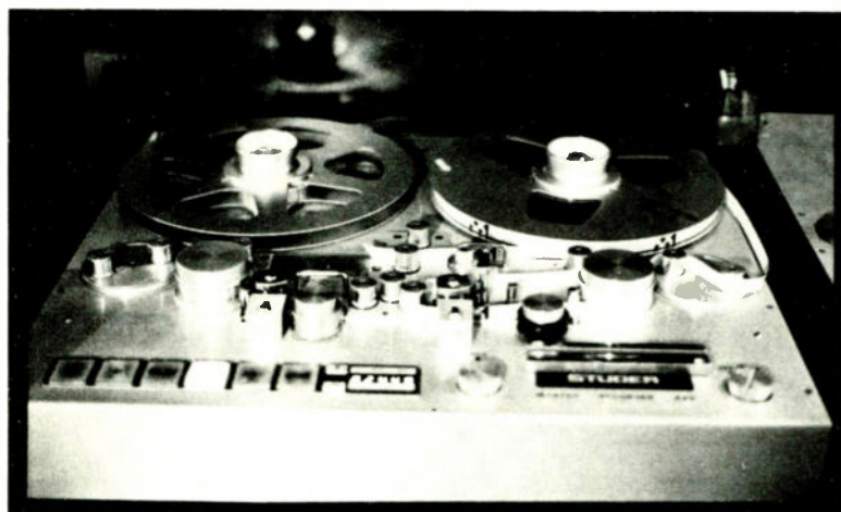
AFTER A SUCCESSFUL CUT: THE "SUPER ANALOG" MASTER TAPE (1/2-INCH, 30-ips, TWO-TRACK STEREO, NO NOISE REDUCTION). MANY POP RECORDS ARE MADE FROM MASTERS IN THIS FORMAT.
