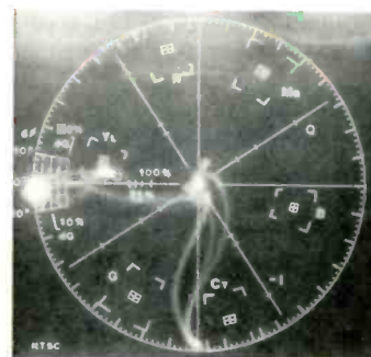
COLOR CONSISTENCY for the VKT-650's recorder section running at the SP speed (left) and for its TV tuner (right). (The results for the VCR in LP and EP are virtually identical to those in SP, so we have omitted the vectorscope photos for the slower speeds.) In each case, the ideal would be for the cluster of dots toward the left edge of the grid to be a single dot at the intersection of the nine-o'clock axis with the circumference. The radial spread of the dots indicates chroma differential gain, which is a measure of how much chroma level (color saturation) varies with changes in scene brightness (luminance). The angular spread shows the chroma differential phase, which tells how much chroma phase (hue) shifts with changes in brightness. Both the tuner and the VCR perform well in this test although the former shows a large differential gain at the highest luminance level.
