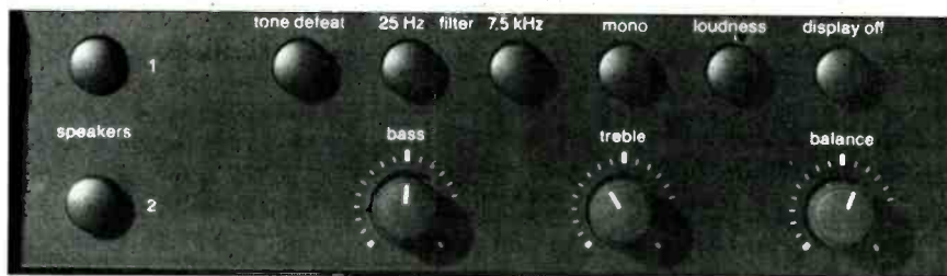
Secondary controls are at the left end of the front panel, behind a flip-down door.
