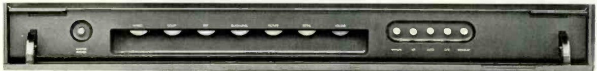
THE PROTON'S MAIN CONTROLS are behind a flip-down door at the bottom of the screen. From left, they are the power switch, VERTICAL HOLD, COLOR, TINT, BLACK LEVEL (brightness), PICTURE (contrast), DETAIL (sharpness), VOLUME (which regulates the output of the 600M's built-in stereo audio amplifier), the three color-control switches (manual, Vertical Interval Reference, and automatic flesh-tone correction), the OPC ("Optimum Picture Control") switch, and the standby (automatic turn-on) switch. The color-control switches are mutually exclusive, but when the set is in VIR and there is no Vertical Interval Reference in the signal, the monitor reverts to the manual settings.
