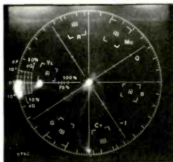
TUNER COLOR CONSISTENCY. The narrow angular spread of the color vectors (the white dots near the periphery of the grid) indicates low chroma differential phase: Hues shift very little with changes in brightness on the SL-2700's tuner. Chroma differential gain, indicated by the dots' radial spread, is not as good. But since the only significant drop in color saturation occurs at the top of the luminance scale, there will be little change in color saturation, except in the brightest scenes.
