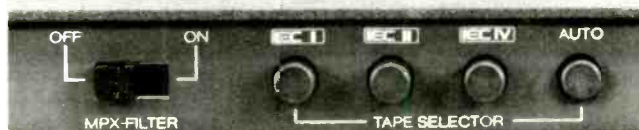
Also behind the door are the multiplex-filter switch and the tape-selector buttons. The latter have positions for IEC types I, II, or IV, or automatic selection based on the keyways in cassette shells.
