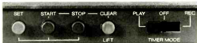
Ordinarily hidden behind the flip-down door at the top of the front panel, these switches control memory stop, memory repeat, and timer-controlled recording and playback.
