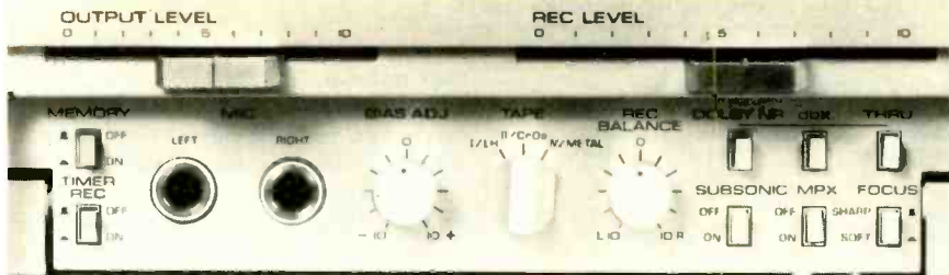
Flip-down panel conceals the K-960's "set-and-forget" controls, which include a tape-type selector, a fine-bias adjustment, a recording balance control, noise reduction selectors (Dolby B or DBX), and Yamaha's unique Focus switch.
