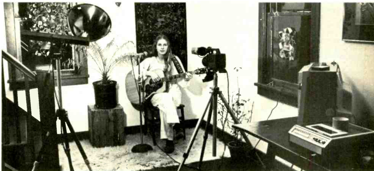
Basic setup (below) included two lights, standard color TV, portable VCR, single-tube color camera, and a quality microphone. Placement of monitor near camera allowed performer to see the image being recorded at any particular moment.
